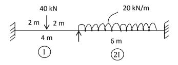
4 Analyze the beam by moment distribution method. The beam at supports B and C sinks by 2 mm and 7 mm. Take E =  $200 \text{ kN/mm}^2$  and I =  $2.5 \times 10^7 \text{ mm}^4$ .
